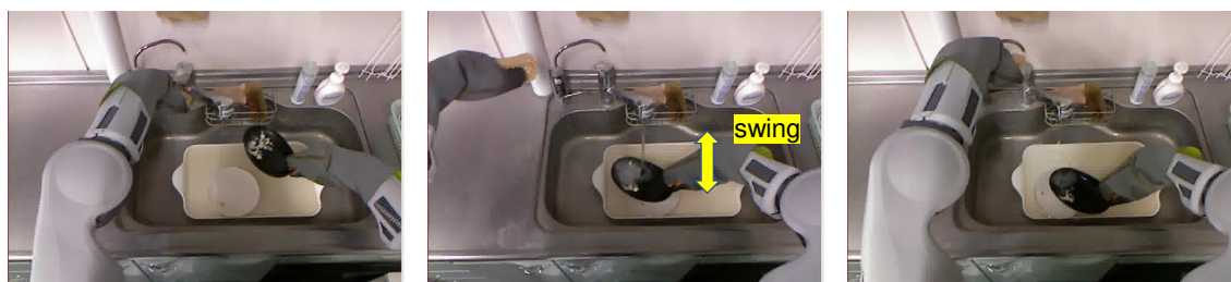
Fig. 6.10: The picture on the left shows the point with dirt on it, which is the target value for the trajectory. The picture on the right shows the dirt detection by image processing.
