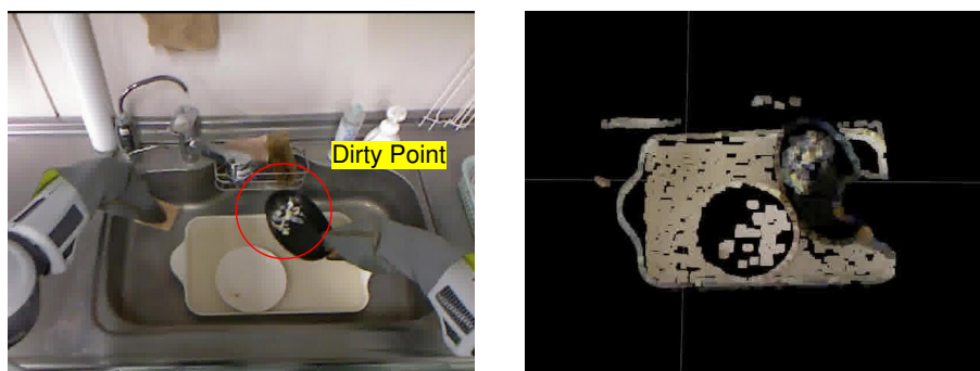
Fig. 6.10: The picture on the left shows the point with dirt on it, which is the target value for the trajectory. The picture on the right shows the dirt detection by image processing.
