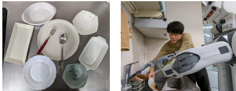
Fig. 6.9: The left picture is the dishes for washing training. The dishes are including various size and shape of plate, fork and spoon. The right picture is the robot training of manipulation taught by human.
