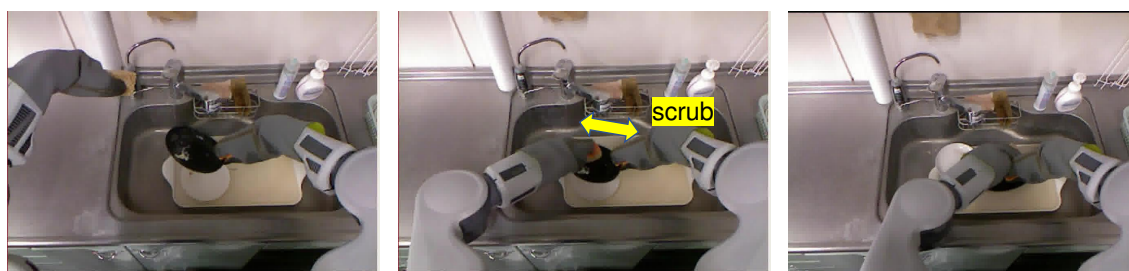
Fig. 6.11: The optimization result of rinsing dish. The robot is rinsing while swaying its arms.
