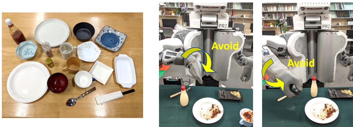
Fig. 6.2: Tableware for training (left). Avoiding obstacles and approaching the rim dish (middle, right). After reaching the object, the robot adjusts its gripper pose.
