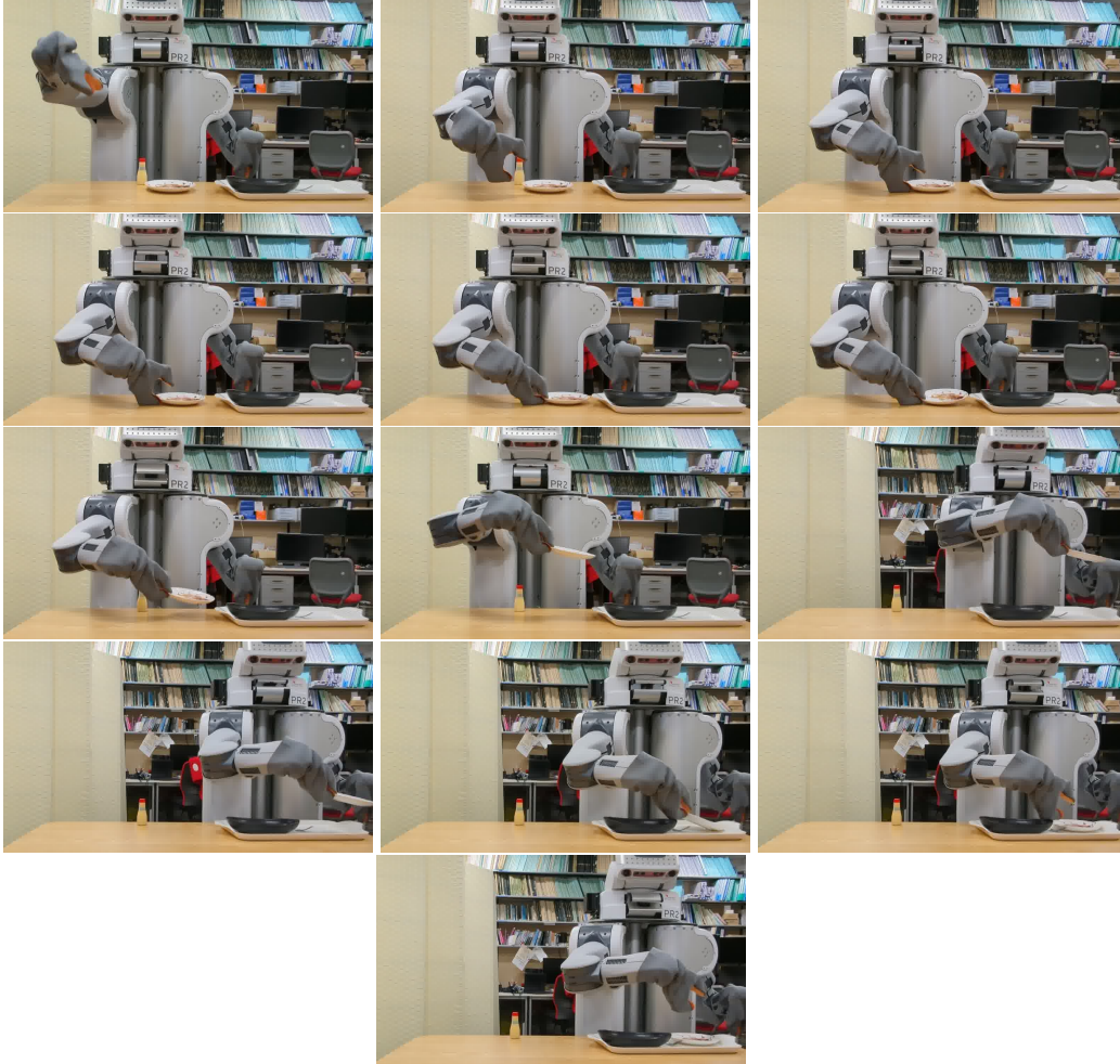
Fig. 6.18: Grasp and put a plate, avoiding the dirt on the front side.
