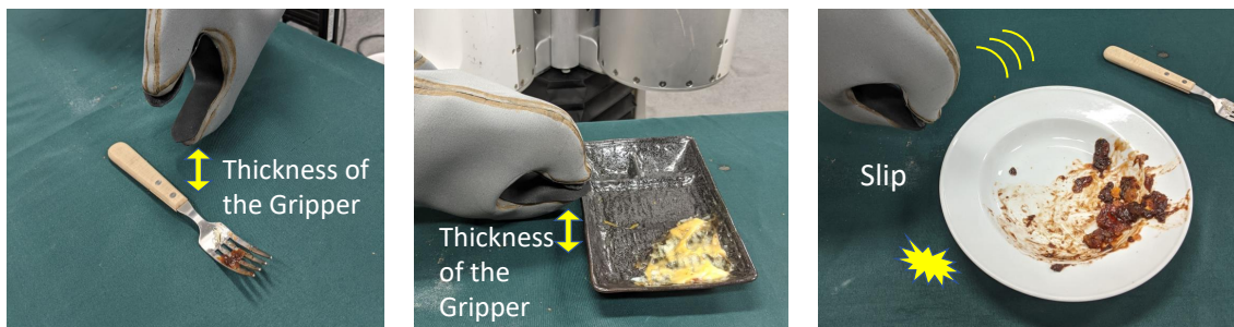
Fig. 6.2: Tableware for training (left). Avoiding obstacles and approaching the rim dish (middle, right). After reaching the object, the robot adjusts its gripper pose.
