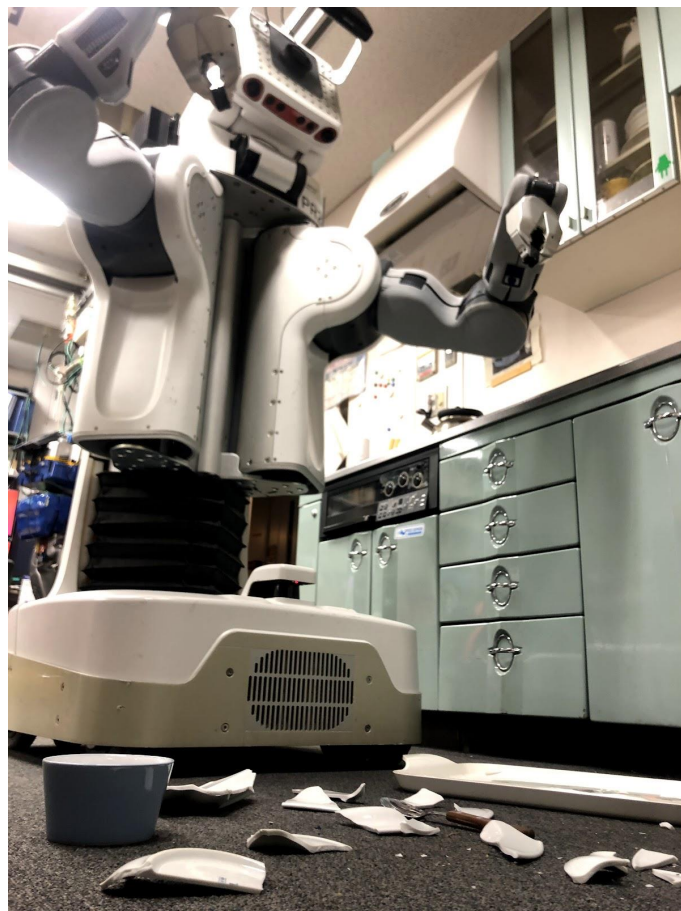
Fig. 6.20: The PR2 drops the tray. Since the tray is instability and the PR2 slips it.
