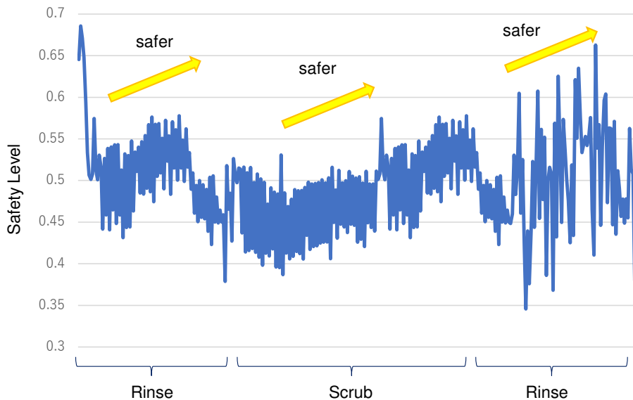
Fig. 6.13: The experimental result of the safety level of the manipulation. The rinsing and scrubbing phases increase the level of safety from its beginning.
